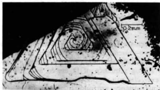
Fig. 6. Optical micrograph of (0001) face of the same crystal (411R and its intergrowth structures) showing four cooperating spiral ledges. All the spirals originate from the centre.
